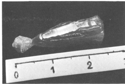
Figure 7 Fresnoite crystal with 20 at.% Si (nominal) with tetragonal (110) faceting (scale in cm).
